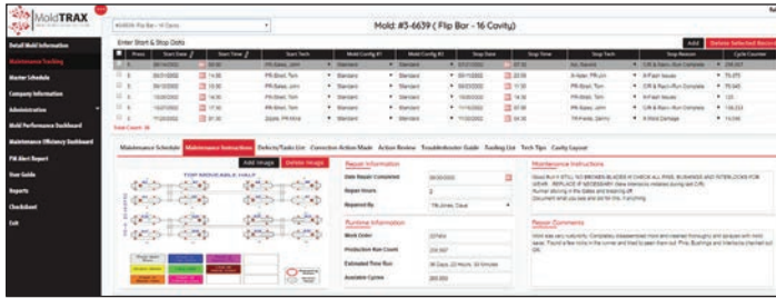
The Maintenance Tracking Section displays mold production run dates and times, press number and stop reasons, along with mold configuration changeovers.
